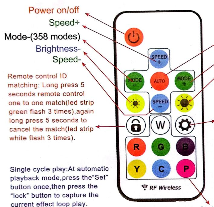
Press the button to play 358 automatically The effect. Press 5 times to enter RGB color jump mode Convenient lamp test.
